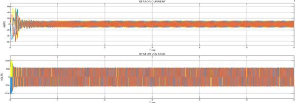
Figure 8: Three phase current and voltage waveforms in system 1 with basic V/F control (constant drive)
