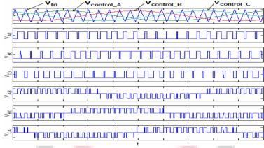
Figure 6: Reference signal generation for PWM
