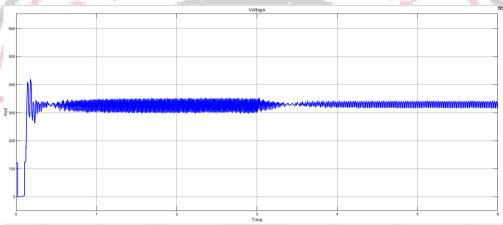
Figure 22: RMS voltage waveform representation in system 1 with basic V/F control (Deceleration mode)
