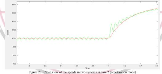
Figure 20 is the comparative graph of speeds in the two systems with closer view of the variations produced in them during acceleration mode. The green graph as shown is having more variable waveform when the speed is increased at 3 sec producing a spike and the red graph is increasingly more smoothly.
