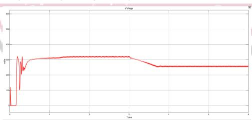
Figure 23: RMS voltage waveform representation in system 2 with parametric ant colony optimization control (Deceleration mode)
