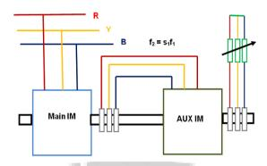
Figure 2: Cascade Operation In Controlling Speed of Induction Motor
